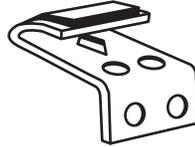
**HB KWIK** – This hook-back, one-staple clip is hooked over the outside of the frame. One staple, either on the top of the frame or on the outside, does the job. Needs no second staple.
